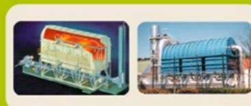
OXYDATION THERMIQUE RÉGÉNÉRATIVE (RTO)
